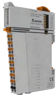
Thermocouple (TC) measurement module, 16 bit resolution, 4 channels
